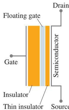
**FIGURE 21-30** A floating gate nonvolatile memory cell (NVM).
