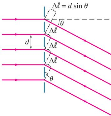
FIGURE 24-24 Diffraction grating.
