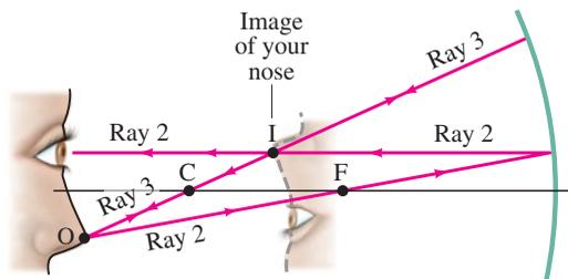
**FIGURE 23–18** You can see a clear inverted image of your face in a concave mirror when you are beyond C ( $d_o > 2f$ ), because the rays that arrive at your eye are *diverging*. Standard rays 2 and 3 are shown leaving point O on your nose. Ray 2 (and other nearby rays) enters your eye. Notice that rays are diverging as they move to the left of image point I.
