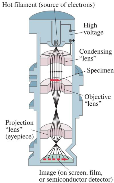
**FIGURE 27-14** Transmission electron microscope. The magnetic field coils are designed to be "magnetic lenses," which bend the electron paths and bring them to a focus, as shown. The sensors of the image measure electron intensity only, no color.
