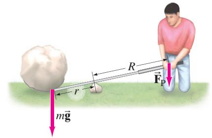
**FIGURE 9–6** Example 9–3. A lever can “multiply” your force.
