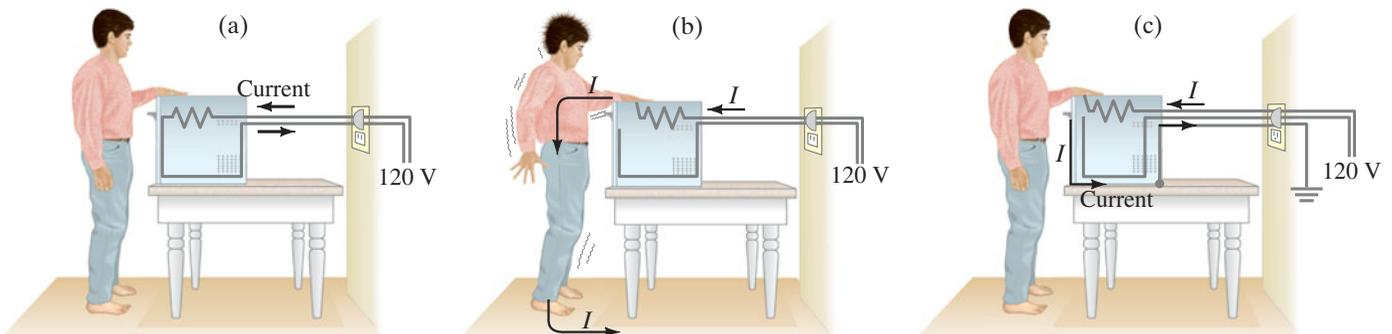
**FIGURE 19–26** (a) An electric oven operating normally with a 2-prong plug. (b) A short to a metal case which is ungrounded, causing a shock. (c) A short to the case which is grounded by a 3-prong plug; almost no current goes through the person.
