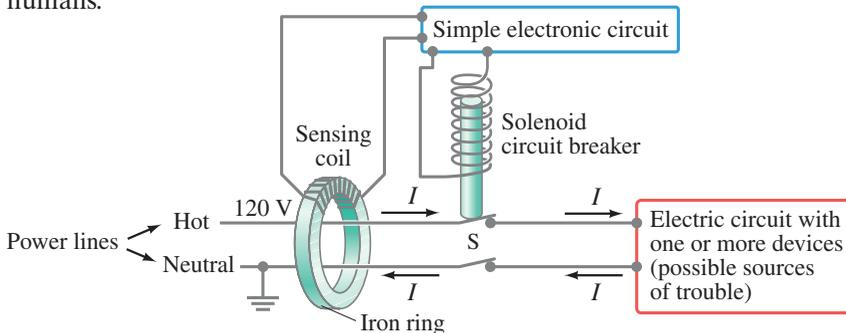
**FIGURE 21-33** A ground fault circuit interrupter (GFCI).
