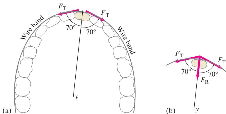
**FIGURE 9–3** Forces on a tooth. Example 9–1.
