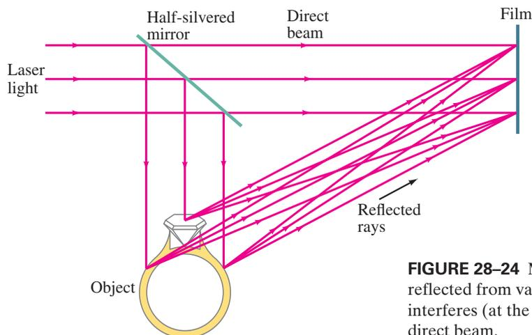
**FIGURE 28–24** Making a hologram. Light reflected from various points on the object interferes (at the film) with light from the direct beam.
