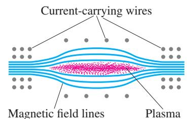
**FIGURE 31-13** “Magnetic bottle” used to confine a plasma.
