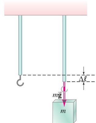
**FIGURE 9–18** Hooke’s law:  $\Delta\ell \propto$  applied force.
