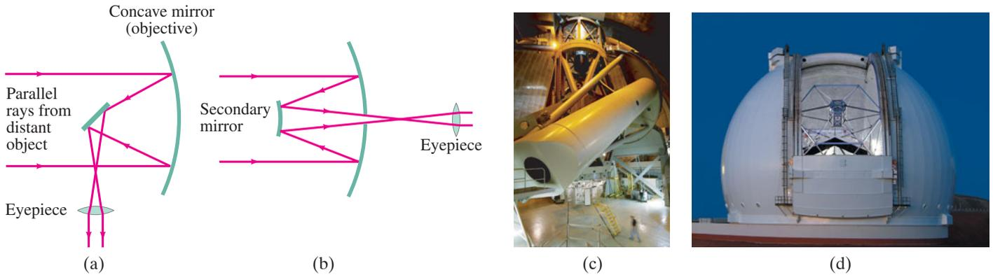
**FIGURE 25–22** A concave mirror can be used as the objective of an astronomical telescope. Arrangement (a) is called the Newtonian focus, and (b) the Cassegrainian focus. Other arrangements are also possible. (c) The 200-inch (mirror diameter) Hale telescope on Palomar Mountain in California. (d) The 10-meter Keck telescope on Mauna Kea, Hawaii. The Keck combines thirty-six 1.8-meter six-sided mirrors into the equivalent of a very large single reflector, 10 m in diameter.
