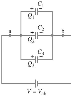
**FIGURE 19-17** Capacitors in parallel:  $C_{\text{eq}} = C_1 + C_2 + C_3$ .
