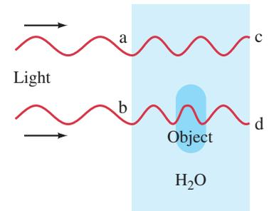
FIGURE 25–34 Object—say, a bacterium—in a water solution.
