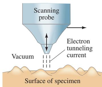
**FIGURE 27-17** The probe tip of a scanning tunneling electron microscope, as it is moved horizontally, automatically moves up and down to maintain a constant tunneling current, and this motion is translated into an image of the surface.
