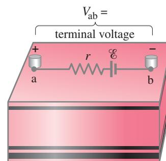
FIGURE 19–1 Diagram for an electric cell or battery.
