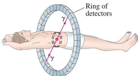
**FIGURE 31–21** Positron emission tomography (PET) system showing a ring of detectors to detect the two annihilation  $\gamma$  rays ( $e^+ + e^- \rightarrow 2\gamma$ ) emitted at  $180^\circ$  to each other.
