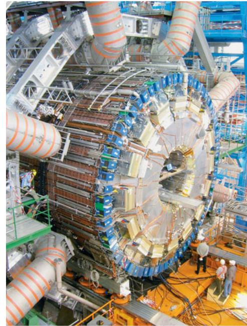
**FIGURE 32–6** ATLAS, one of the large complex detectors at the LHC, is shown here as it was being built. In 2012 it was used to provide evidence for the Higgs boson. Note the people near the bottom. From the outside, the CMS detector at the LHC looks similar.
