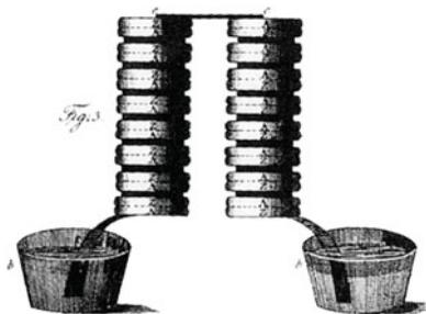
**FIGURE 18–2** A voltaic battery, from Volta's original publication.
