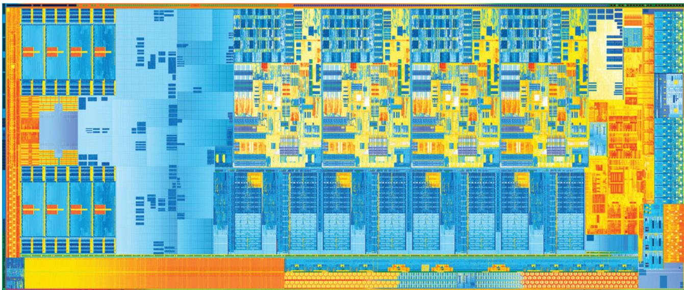
This computer processor chip contains over 1.4 billion transistors, plus diodes and other semiconductor electronic elements, all in a space of about  $1\text{ cm}^2$ . It uses 22-nm technology, meaning the “wires” (conducting lines) are 22 nm wide.
