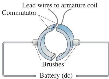
**FIGURE 20–38** Commutator-brush arrangement in a dc motor ensures alternation of the current in the armature to keep rotation continuous in one direction. The commutators are attached to the motor shaft and turn with it, whereas the brushes remain stationary.
