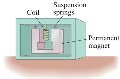
**FIGURE 21-32** One type of seismograph, in which the coil is fixed to the case and moves with the Earth's surface. The magnet, suspended by springs, has inertia and does not move instantaneously with the coil (and case), so there is relative motion between magnet and coil.
