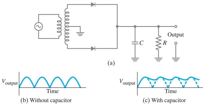
**FIGURE 29-32** (a) Full-wave rectifier circuit (including a transformer so the magnitude of the voltage can be changed). (b) Output voltage in the absence of capacitor  $C$ . (c) Output voltage with the capacitor in the circuit.
