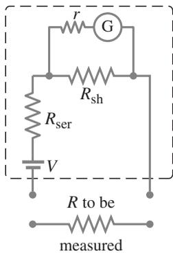
FIGURE 19–35 An ohmmeter.
