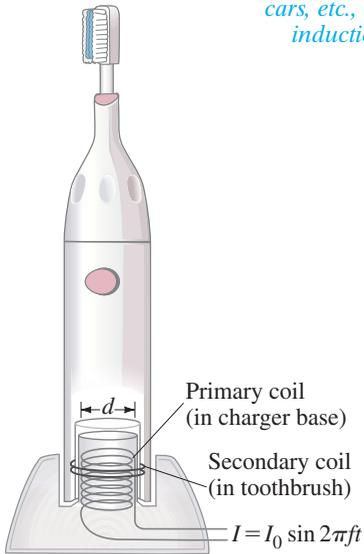
**FIGURE 21–26** This electric toothbrush contains rechargeable batteries which are being recharged as it sits on its base. Charging occurs from a primary coil in the base to a secondary coil in the toothbrush. The toothbrush can be lifted from its base when you want to brush your teeth.
