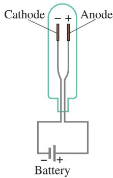
**FIGURE 17–28** If the cathode inside the evacuated glass tube is heated to glowing (by an electric current, not shown), negatively charged “cathode rays” (= electrons) are “boiled off” and flow across to the anode (+), to which they are attracted.
