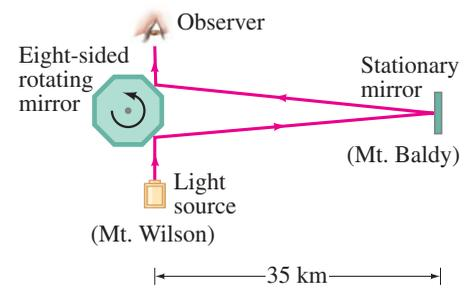
FIGURE 22–10 Michelson's speed-of-light apparatus (not to scale).
