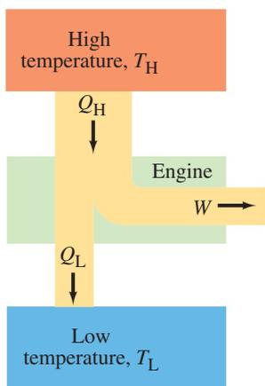
**FIGURE 15-11** Schematic diagram of energy transfers for a heat engine.
