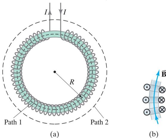
**FIGURE 20-60** Problem 49. (a) A toroid or torus. (b) A section of the toroid showing direction of the current for three loops:  $\odot$  means current toward you, and  $\otimes$  means current away from you.
