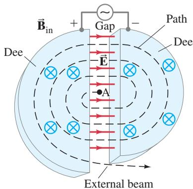
**FIGURE 32-2** Diagram of a cyclotron. The magnetic field, applied by a large electromagnet, points into the page. The protons start at A, the ion source. The red electric field lines shown are for the alternating electric field in the gap at a certain moment.
