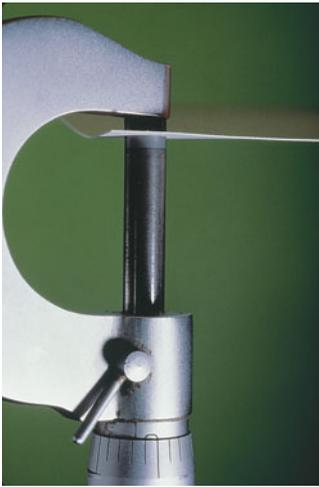
**FIGURE 1-11** Example 1-7. Micrometer used for measuring small thicknesses.
