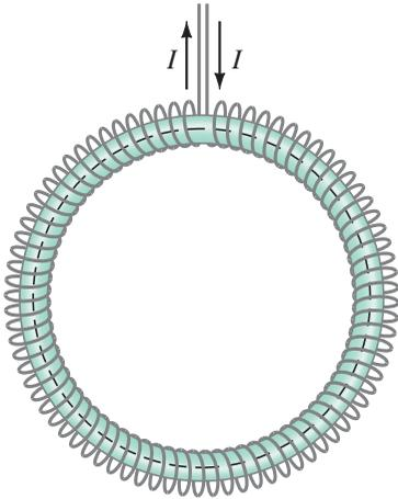
FIGURE 20–44 Iron-core toroid.
