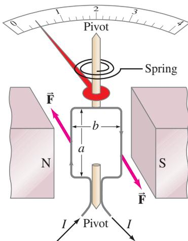
FIGURE 20–35 Galvanometer.
