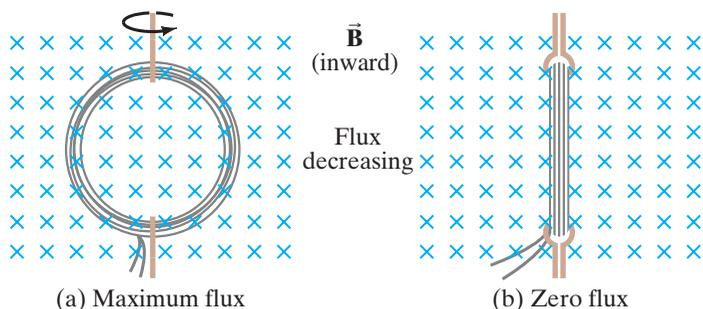
**FIGURE 21–6** A current can be induced by rotating a coil in a magnetic field. The flux through the coil changes from (a) to (b) because  $\theta$  (in Eq. 21–1,  $\Phi = BA \cos \theta$ ) went from  $0^\circ$  ( $\cos \theta = 1$ ) to  $90^\circ$  ( $\cos \theta = 0$ ).
