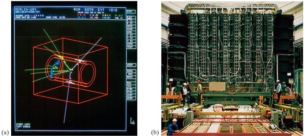
**FIGURE 32-10** (a) Computer reconstruction of a Z-particle decay into an electron and a positron ( $Z^0 \rightarrow e^+ + e^-$ ) whose tracks are shown in white, which took place in the UA1 detector at CERN. (b) Photo of the UA1 detector at CERN as it was being built. 1980s.
