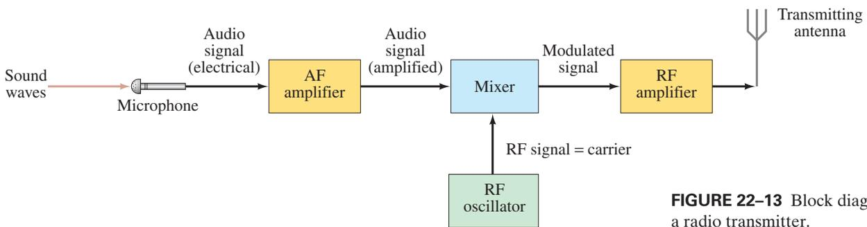
**FIGURE 22–13** Block diagram of a radio transmitter.
