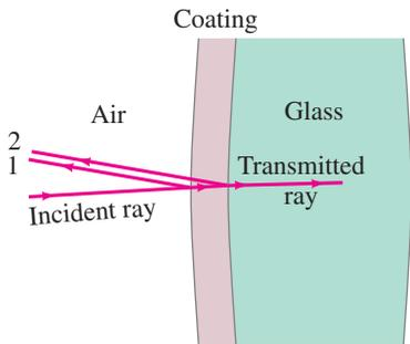
**FIGURE 24–36** Lens coating, Example 24–12. Incident ray of light is partially reflected at the front surface of a lens coating (ray 1) and again partially reflected at the rear surface of the coating (ray 2), with most of the energy passing through as the transmitted ray into the glass.
